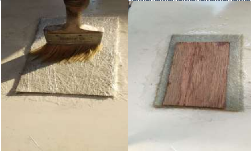
Fig 2. Application of epoxy on chopped Fig.3 Plywood placed on the glass fiber sheet Glass fiber sheet
